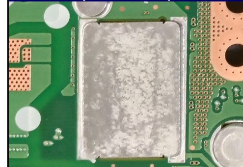
放熱対策(基板裏) Heat dissipation measures (Back side)
